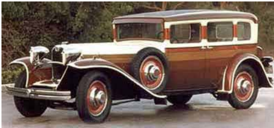
The front-wheel-drive Ruxton was developed by a team of Budd engineers and shown to the public in 1929.
