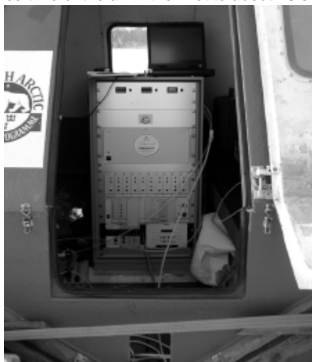
Fig. 1. The PTR-MS instrument was housed in a heated ice hut in a position close to the base station and winch of the TLS.
