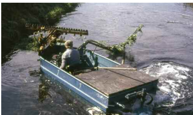
Mowing boats equipped with cutting bars in front and on the side.
