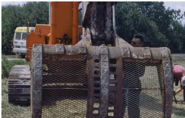
A bucket designed for the mechanised uprooting of water primrose.
