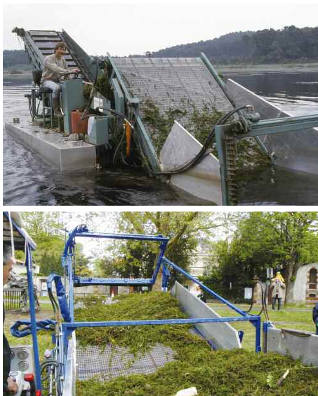
Harvester with the cutting bars and the conveyor belt used to extract the plants from the water.
