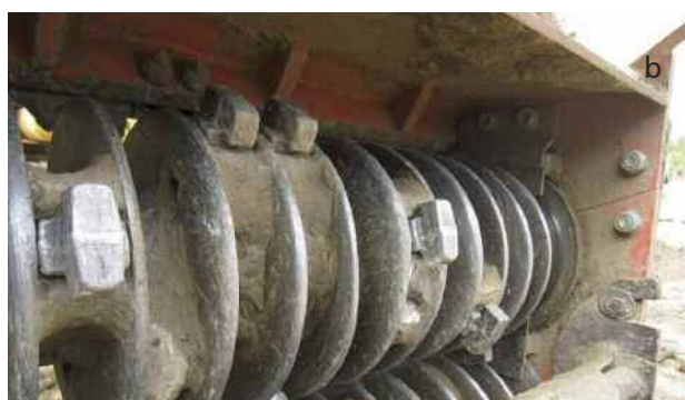
Mechanised management of knotweed in the Gard department, a) soil grinding, b) grinding rotor in the bucket.
