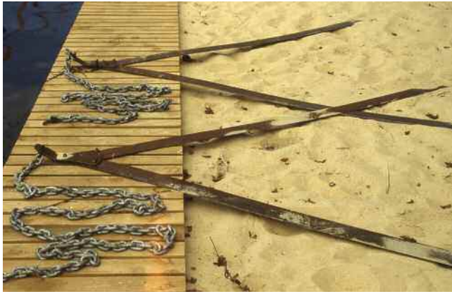
Cutting bar that is dragged along the bottom by a boat.
