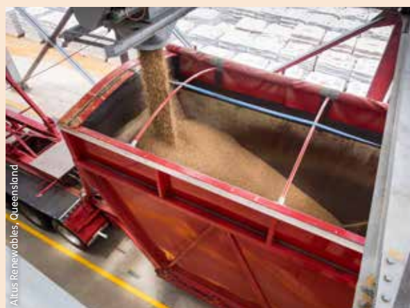
Fuel pellets made from softwood processing residues being loaded onto a truck for transport to the port of Bundaberg, Queensland, from where they are exported to European and Asian markets.
