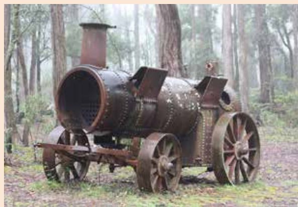
Figure 6.32: Boiler used to power machinery for cutting timber, Lowden Forest Park, New South Wales
