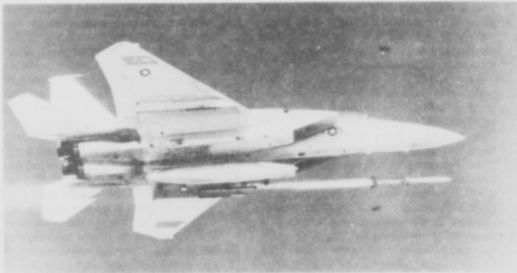
Advanced medium-range air-to-air missile (AMRAAM) test shot from the F-15. The AMRAAM is an important advance over other medium-range radar missiles for several reasons. It is smaller and lighter, jam resistant, and is a fire-and forget weapon. It will be used also on a large part of the F-16 fleet that does not yet have a radar missile capability.
