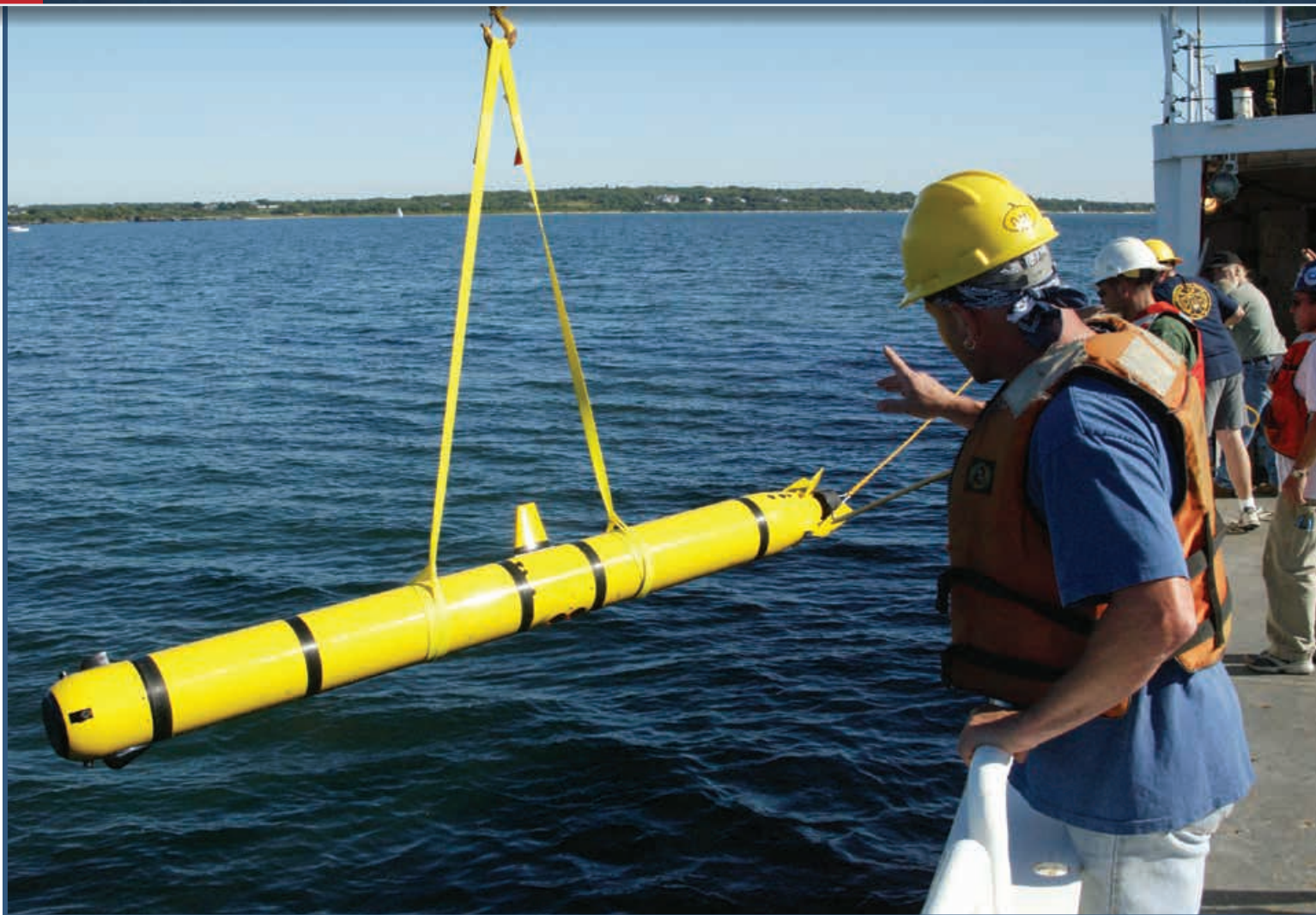
In 2005, the Midsize Autonomous Research Vehicle (MARV), the size of a lightweight torpedo, was tested aboard the University of Rhode Island's R/V Endeavor. From torpedoes to autonomous vehicles, NUWC Division Newport is focused on advancing the state of art of undersea warfare and meeting the needs of the U.S. Navy fleet.
