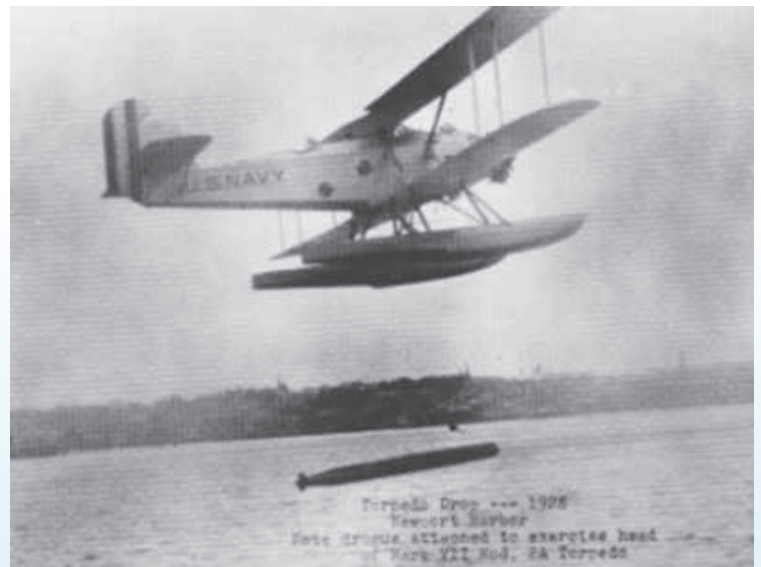
This 1925 photo shows a torpedo drop in Narragansett Bay from a plane assigned to the Station Air Detail on Gould Island. Note the drogue attached to the exercise head of a Mark VII torpedo. (Photo courtesy Naval War College Museum)
