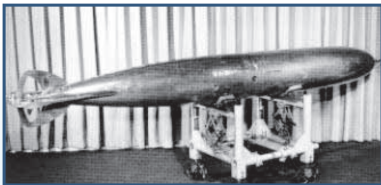
The brass Howell torpedo (Fish type) was the first automobile torpedo issued to the fleet. Its range was 400 yards at a speed of 25 knots (maximum range 700 yards) and the warhead charge was 100 pounds of guncotton. Just prior to launching, a 130-pound flywheel was spun to 10,000 rpm by a ship-mounted steam engine. (Photo courtesy Naval War College Museum)
