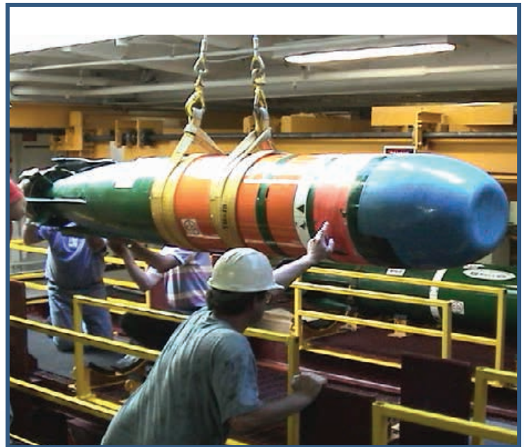
In 2002, the Advanced Half Length Torpedo was part of the Swampworks portfolio of rapid-response technology insertions sponsored by the Office of Naval Research (ONR) and developed by NUWC Division Newport. The torpedo included a high-frequency, littoral sonar added to the ADCAP sonar for improved target discrimination in noisy littoral environments. Swampworks efforts focused on a set of high-risk, high-payoff programs to respond to both emerging and enduring fleet operational challenges. The half-length requirement allowed twice as many torpedoes to be carried and improved flexibility in loading-out for other missions. (Source: NUWScope, October 2002)
