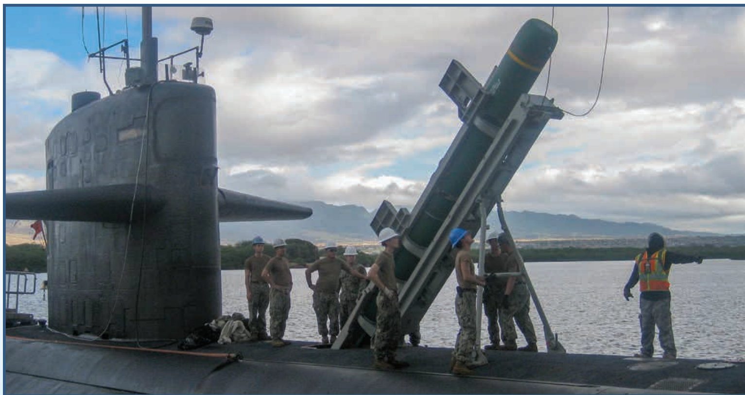
Sailors load a Harpoon anti-ship cruise missile onto the Los Angeles-class fast-attack submarine USS Olympia (SSN-717) as part of the biannual Rim of the Pacific Exercise, July 3, 2018. (U.S. Navy photo/released)
