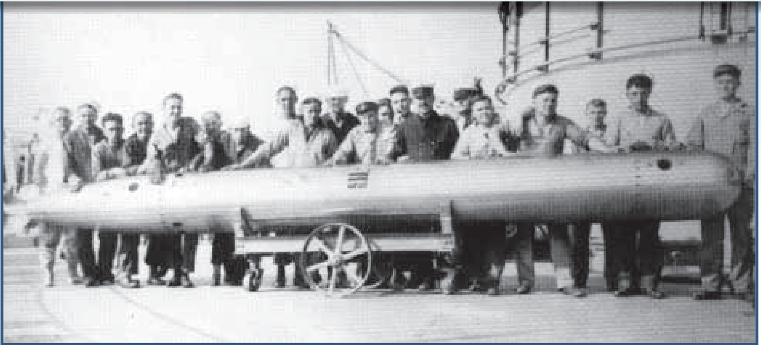
The Mark 9 weapon was a Bliss-Leavitt torpedo developed and produced by the E. W. Bliss Co. and Naval Torpedo Station in Newport. It was designed in 1915 for use on battleships. Later, the Mark 9 was modified for use on submarines.
