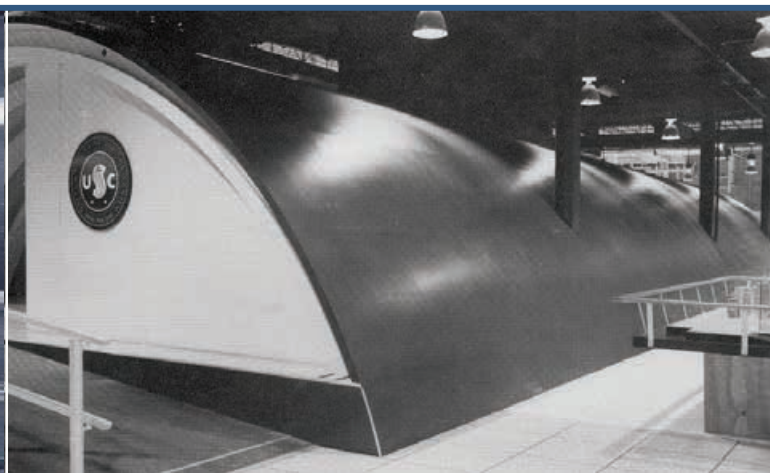
Developed in the 1980s, this test bed was a full-scale submarine mockup for combat system operational evaluation. It was used for both near-term and advanced concepts. Views of the internal (left) and external (right) test setup are shown.
