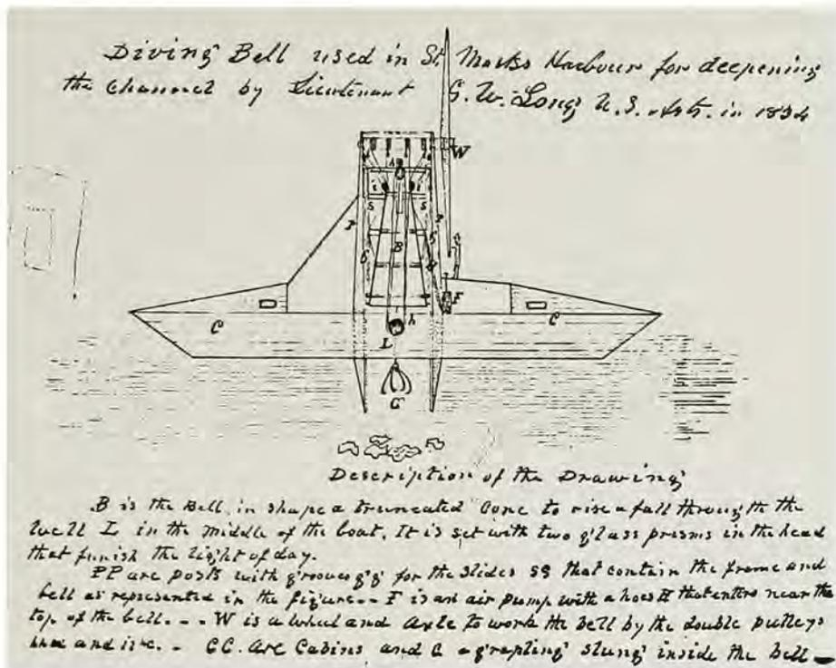
readied their load, the wheel and axle was employed, which raised the diving rig high enough in the ship's well for a platform to be slid under the bell to remove the stone in the grapple. Then the whole performance would be repeated.<sup>37</sup>
