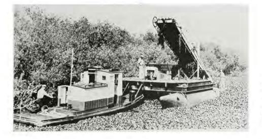
Conveyor system pulls Hyacinths into shredder on Lake Okeechobee, March 1973 when Corps of Engineers conducted crash spraying program. Courtesy Corps of Engineers.
