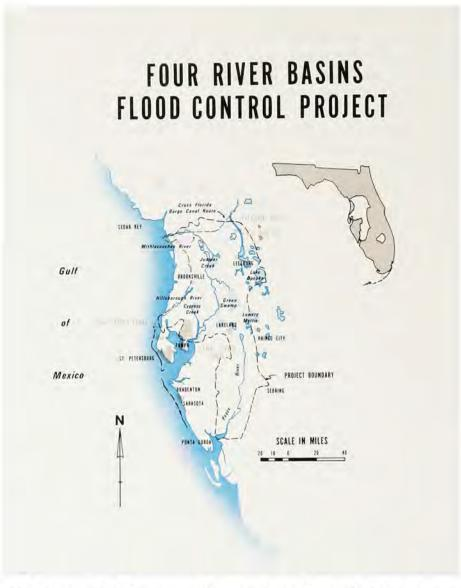
will be connected by many miles of channels, protected by levees and other water control structures. Lake Apopka will have a levee along its north shore while other devices are planned for Peace River, Lake Tarpon, Anclote River, and Pithlachascotee River.
