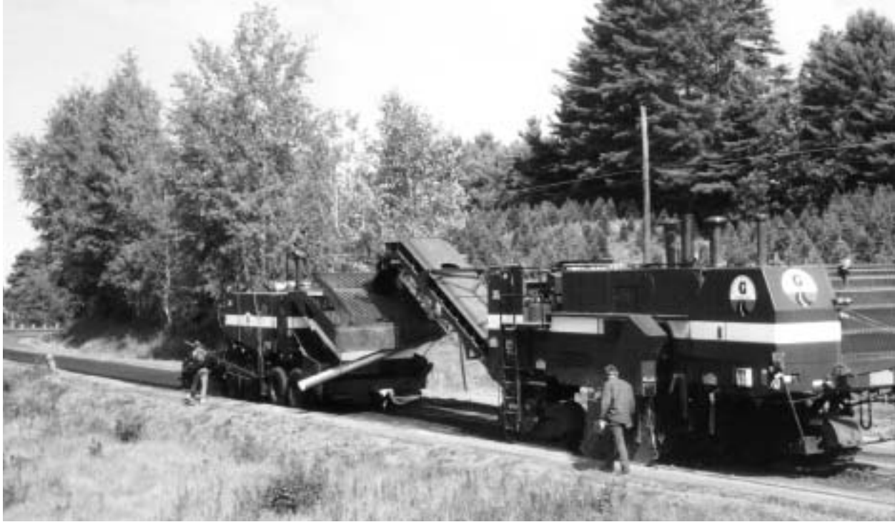
Figure 17-3: Cold Recycling Paver with Integral Pugmill. Microprocessor controlled aggregate and emulsion measuring systems provide accurate proportioning.
