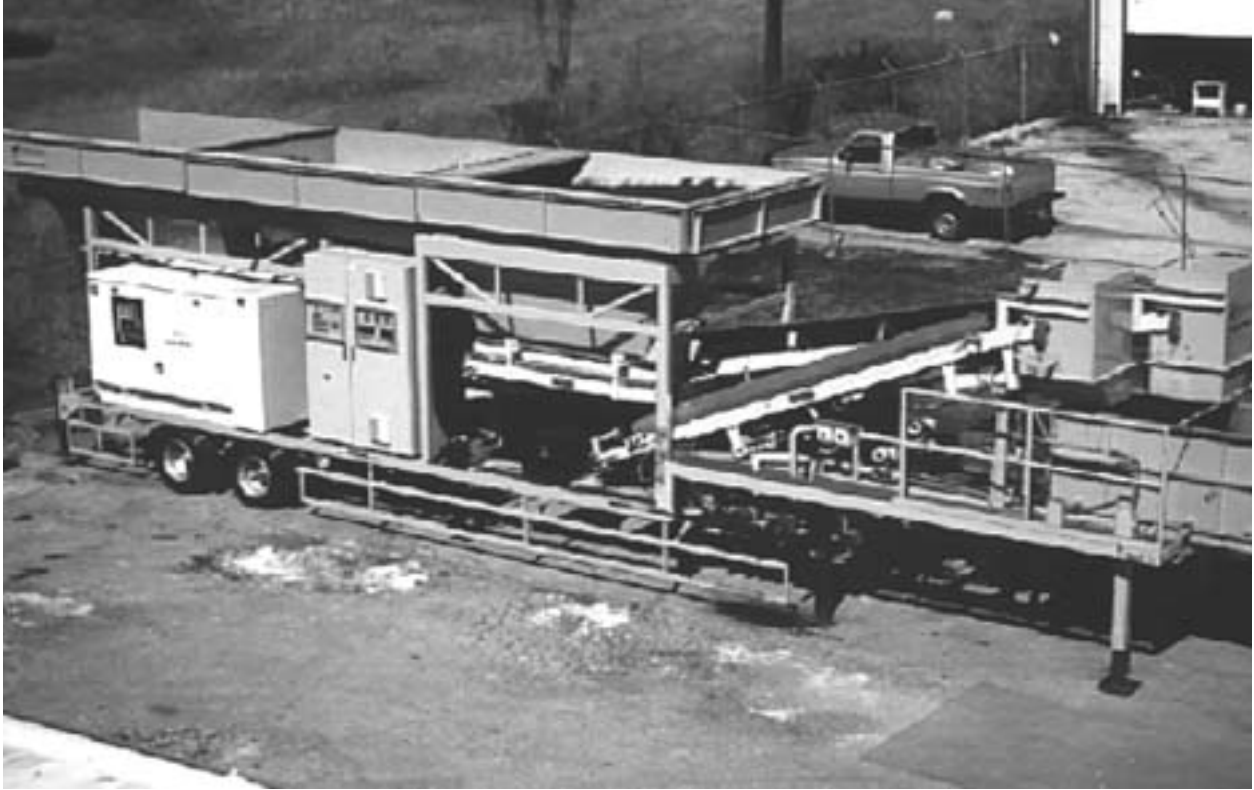
Figure 16-11: Conventional CCPR plant
