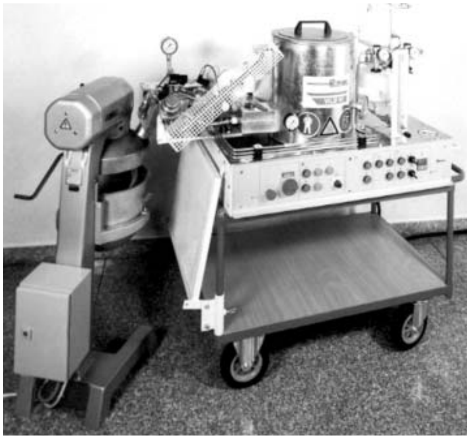
Figure 11-5: Laboratory Asphalt Foaming Plant
