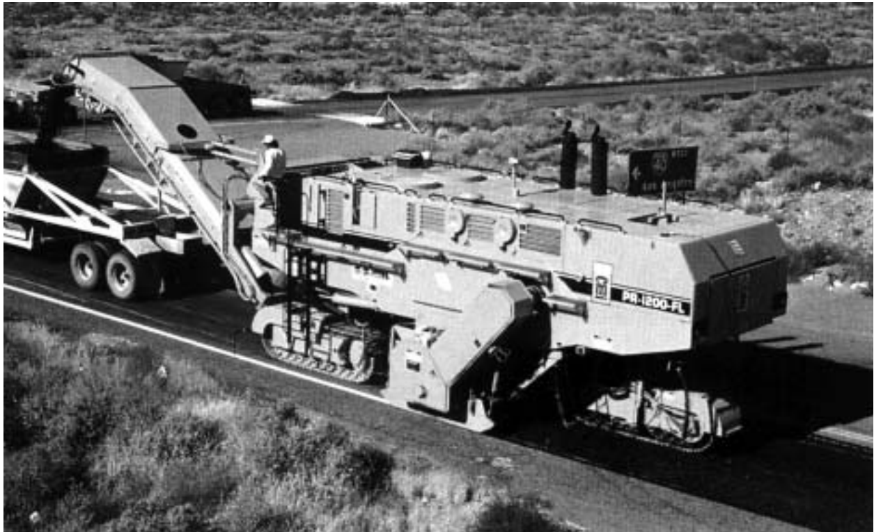
Figure 8-2: High capacity full lane cold planer
