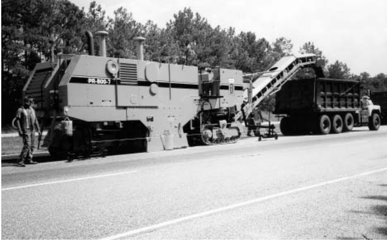
Figure 1-2: Typical front loading milling machine
