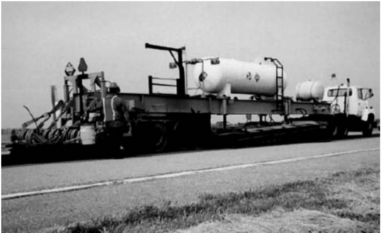
Figure 6-2: Heating and scarifying unit
