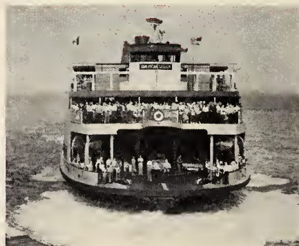
The Staten Island Ferry, "American Legion," built and launched about a year ago in Texas, is now at work in New York Harbor's Upper Bay where she transports passengers across the five-mile distance from the island of Manhattan to Staten Island. The vessel is capable of carrying about 3,500 passengers and 50 cars.
