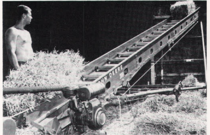
Back in the days of crewcuts, the K-161 Kohler engine was a popular power source on the farm.
