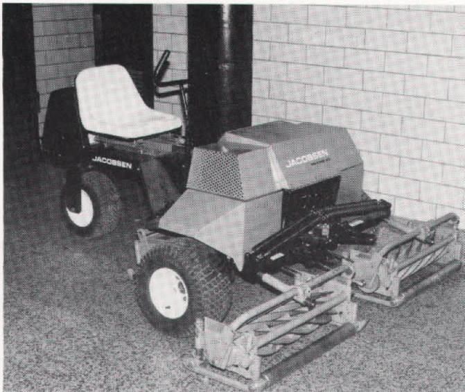
Kohler Magnum 14-HP engine drives Jacobsen's three-gang mower.
