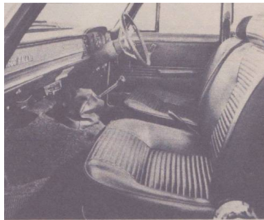
Above. The interior of the Rallye; Note the headrests, the fully adjustable front seats and the centre-mounted handbrake.
