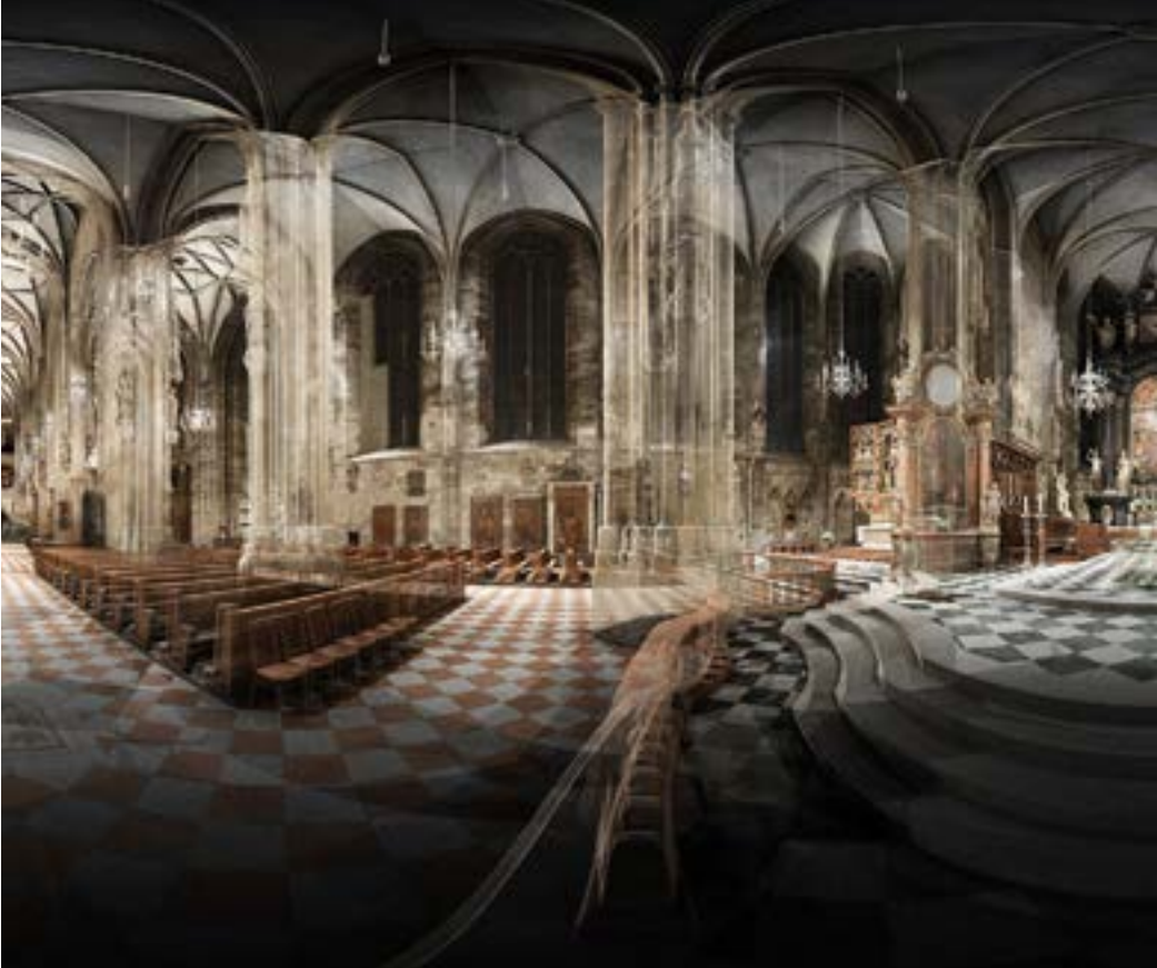
The translucent St. Stephen's Cathedral (2020), St. Stephen's Cathedral in Vienna was spatially measured with more than 20 billion laser points. At this unique level of detail, they correspond to a data volume of almost 400 gigabytes and form the basis of The Translucent St. Stephen's Cathedral ,
