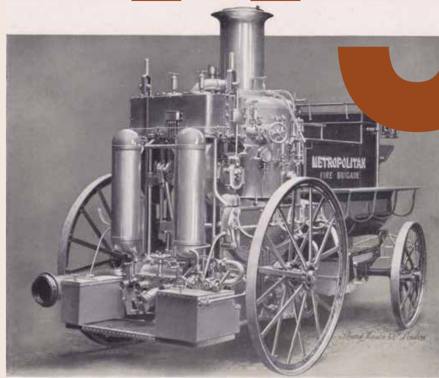
Shand, Mason & Company fire pumps of the day were horse drawn and steam powered. Photo DFES Collection.
