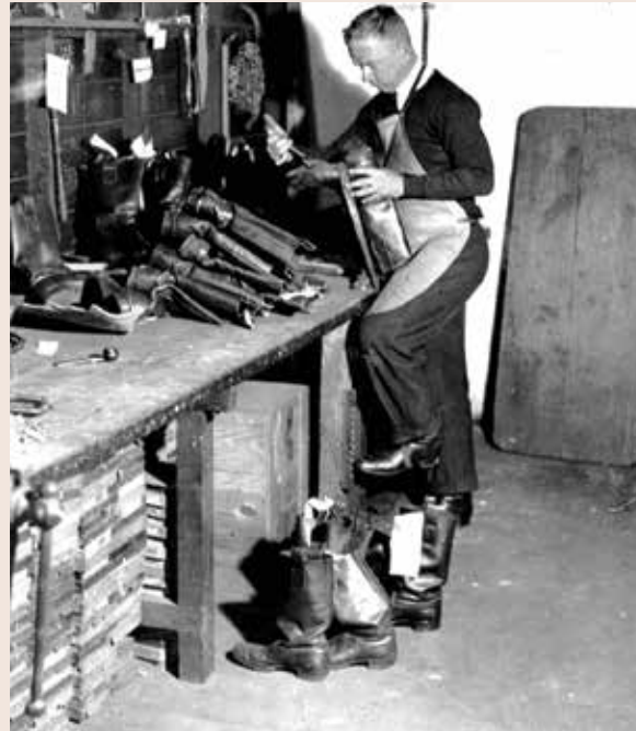
Bootmaker/fireman repairing firemen's boots in workshop area. Photo DFES Collection.
