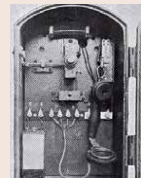
Mobile phone carried by firemen and used to plug into a street alarm box to communicate with fire station. Photo DFES Collection.
