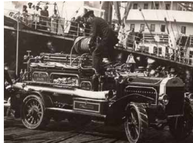
Motorised Dennis Gwynne Pump, first motorised appliance purchased by the WAFB Board. Photo DFES Collection.
