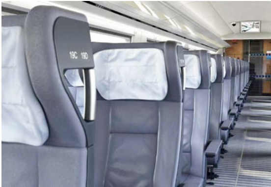
Handholds on the seats, a tactile guidance system with seat numbering in Braille, and strips on the vehicle floor ensure passenger safety and guidance when boarding and while the train is underway.
