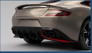
New carbon fibre 2x2 twill rear diffuser and quad exit exhaust tailpipes with optional painted graphics pack
