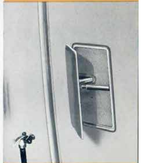
Screened Side Cowl Ventilator
