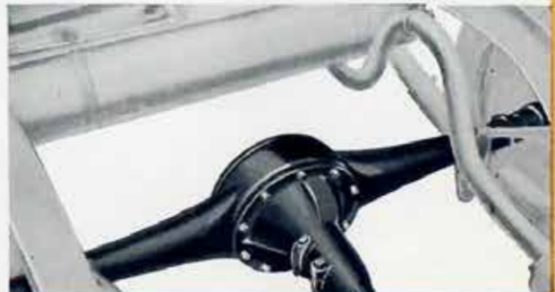
One-Piece Rear Axle Housing
