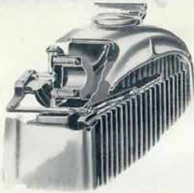
Radiator Shutter Thermostat
