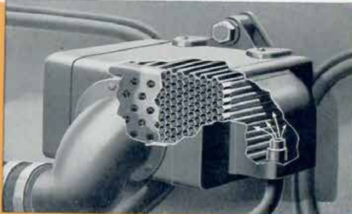
Exclusive Buick Engine Oil Temperature Regulator—Story Page 9
