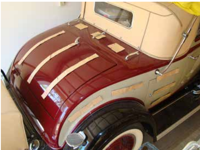
Dynamat Xtreme Damper Pads stop trunk deck and body panel vibration.
