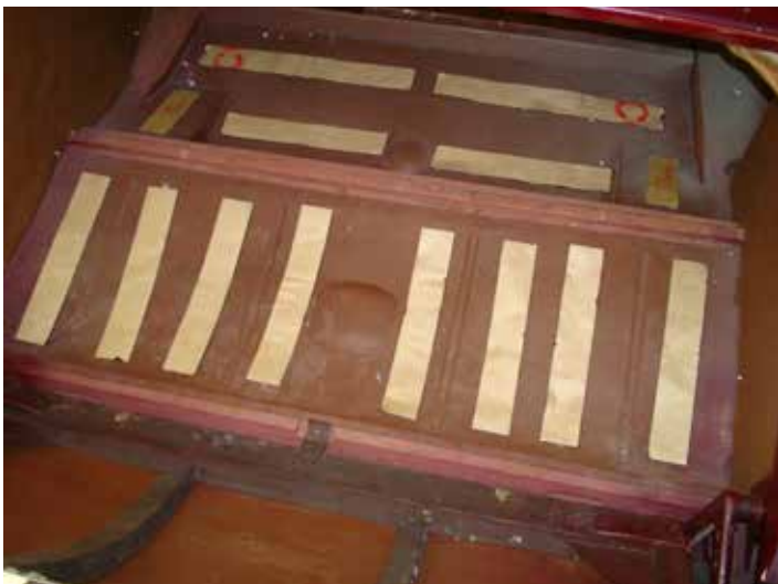
Dynamat Xtreme Damper Pads stop floor panel vibration.
