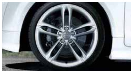
Audi exclusive cast aluminium wheels in 5-parallel-spoke star design size 9 J x 19 with 255/35 R 19 tyres*. From quattro GmbH
