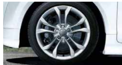
Cast aluminium wheels in 5-parallel-spoke S design size 9 J x 18 with 245/40 R 18 tyres*, optionally available with run-flat tyres
