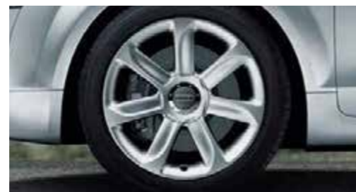
Cast aluminium wheels in 7-arm dynamic design size 9 J x 18 with 245/40 R 18 tyres*, only with run-flat tyres
