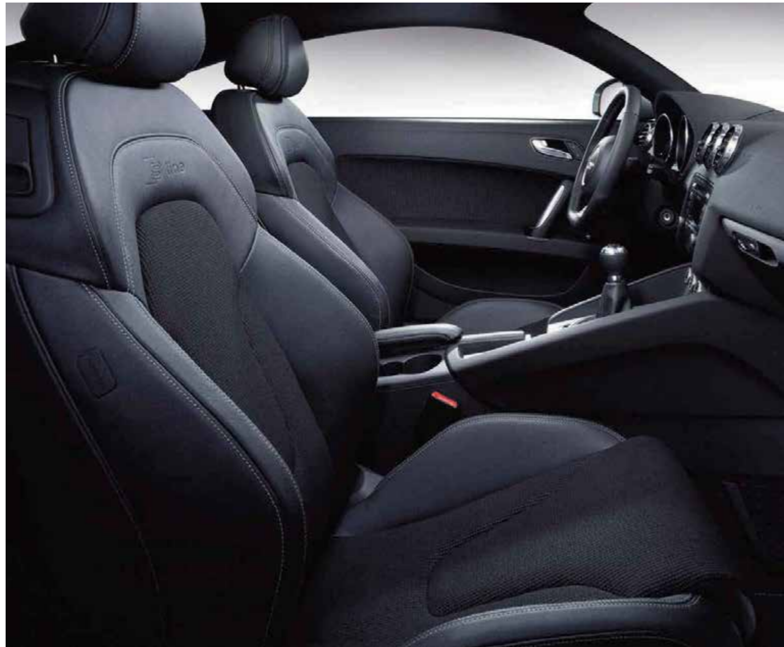
Visibly ergonomic: sport seats, seat upholstery with seat side bolsters in black leather and seat centre panels in black sprint cloth with contrasting stitching and S line embossing on front-seat backrests
