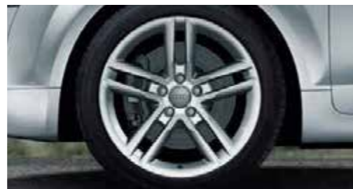
Audi exclusive cast aluminium wheels in 5-twin-spoke design size 9 J x 18 with 245/40 R 18 tyres*. From quattro GmbH
