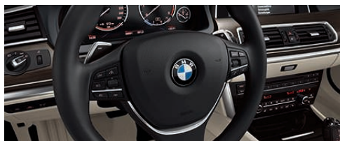
□ Sport leather steering wheel with gearshift paddles . Gears can be changed manually using the paddles mounted on the steering wheel (gearshift paddles only in conjunction with Steptronic transmission with gearshift paddles).
