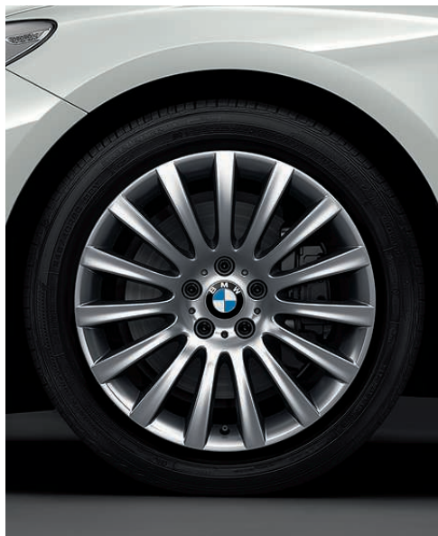
□ 19" light alloy wheels Multi-spoke 235 with mixed tyres. Front: 8.5 J x 19 with 245/45 R 19 tyres. Rear: 9.5 J x 19 with 275/40 R 19 tyres.
