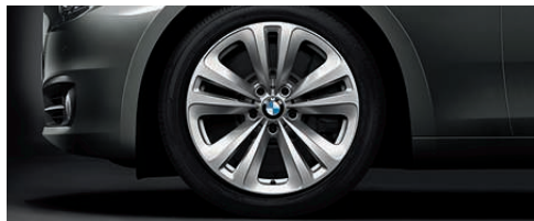
■ 18" light alloy wheels Double-spoke 234 , 8J x 18 with 245/50 R 18 tyres (standard for 535i, 520d, 530d, 535d).
