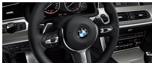
□ M leather steering wheel with gearshift paddles . Gears can be changed manually using the paddles mounted on the steering wheel (gearshift paddles only in conjunction with Steptronic transmission with gearshift paddles).
