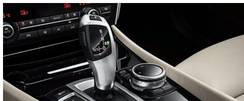
■ Eight-speed Steptronic transmission for significantly faster shift speeds and driving comfort thanks to closely defined gear ratios and smooth transitions. Along with the increase in comfort and dynamism, fuel consumption is also reduced. Additionally, manual shifts can be made via the gearlever.
