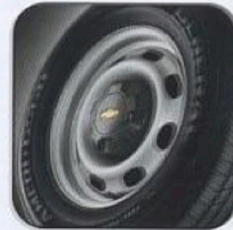
15" x 6" steel wheel, painted gray. Standard on Base models with Z85 Standard suspension.
