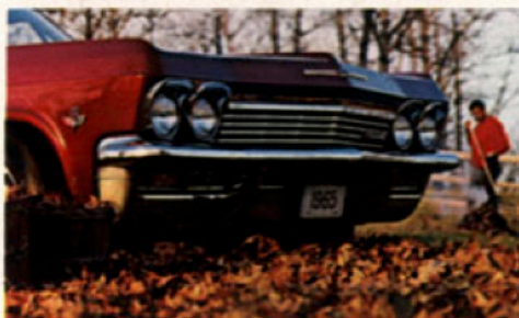
Stylish grille sports Chevrolet nameplate, and a new bumper design protects front body corners.
