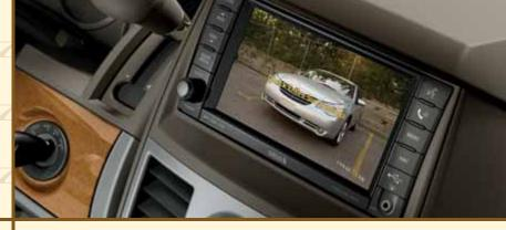
The available ParkView<sup>®</sup> Rear<sup>®</sup> Back-Up Camera<sup>(2)</sup> displays an accurate visual reference of what is behind your vehicle when you are driving in Reverse. Available ParkSense® Rear Park Assist System<sup>(2)</sup> uses audio and visual warnings to assist drivers during reverse parking maneuvers to avoid colliding with most large stationary objects.
