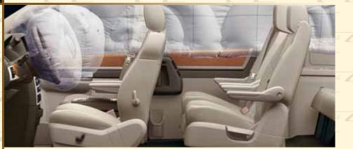
Standard advanced multistage driver and front-passenger air bags<sup>(3)</sup> provide nearly instantaneous front-seat occupant impact protection by matching air bag output to crash severity. Standard supplemental side-curtain air bags<sup>(3)</sup> with rollsensing technology deploy from the headliner to provide three rows of side-impact protection to all outboard passengers. This technology also keeps air bags deployed longer in the
