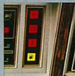
Warning light module—lights for low oil pressure, low voltage, high engine temperature, and low fuel.
