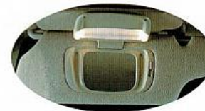
When the engine is switched off, a battery saver switches off the interior lights after 40 minutes should a door be left ajar.
