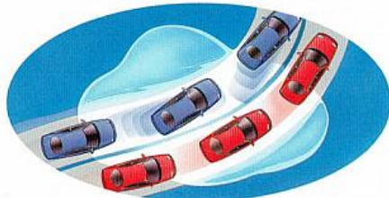
The anti-lock braking system (ABS) is designed to help you maintain steering control in emergency braking situations.
