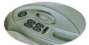
The power windows may be operated for 45 seconds after the ignition has been switched off.
