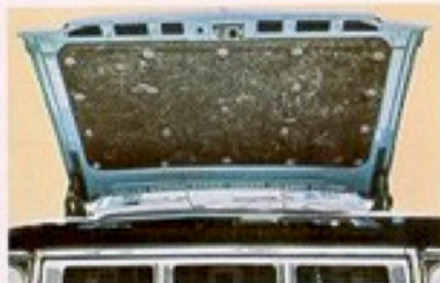
New Hood Design uses dual panels welded together for improved rigidity and reduced hood flutter. Hood insulation (shown above) is available as part of the Sierra or Sierra Grande packages for added sound suppression.
