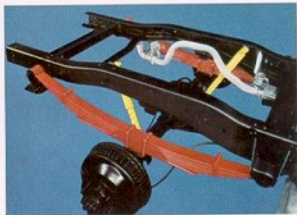
Two-stage leaf spring rear suspension is standard on all light duty models for improved ride control and roll stability. Rear shock absorbers are staggered for improved ride control and to dampen out brake and power hops. Springs and shock absorbers complement each other for improved handling and ride control. New exhaust system hangers permit expansion and contraction of exhaust pipes in operation. New finned cast iron-steel rear brake drums improve cooling.
