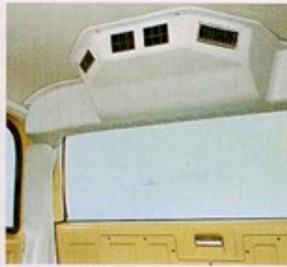
Dual Suburban Air Conditioning adds to driving comfort. Rear unit shown cools and recirculates inside air pre-cooled by front air conditioner. Front air conditioner uses outside or inside air as desired. Ask your GMC dealer for details.
