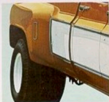
Dual Rear Wheels are available for nominally-rated one-ton Wide-Side models for camper and utility operation. Fiber glass reinforced plastic wheelhouse extensions with front and rear clearance lights are fitted to the standard Wide-Side body. Provide added stability under rough operating conditions.
