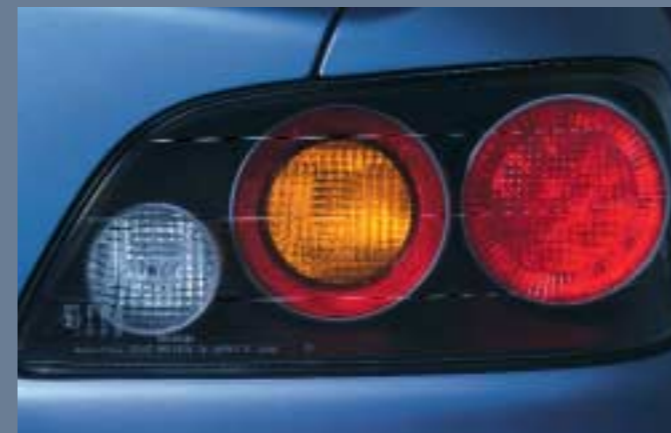
High intensity LED rear brake lights sit with the reversing and driving lights behind impact resistant aerodynamic covers.
