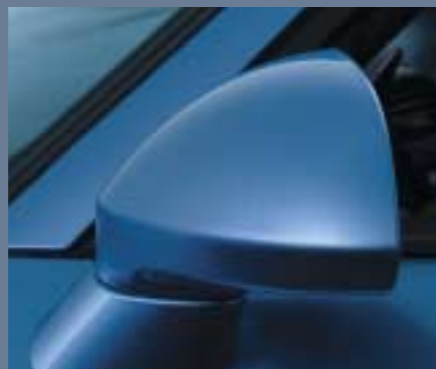
You'll love to drive the Honda S2000 even when the sun's not shining, so the mirrors have heated elements behind the glass to improve rear visibility.
