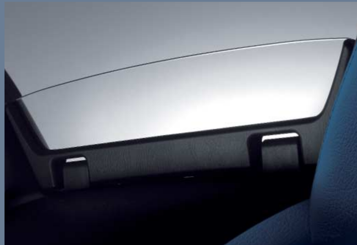
Turbulence in the cabin is reduced, thanks to the folding wind deflector, located between the rear headrests.
