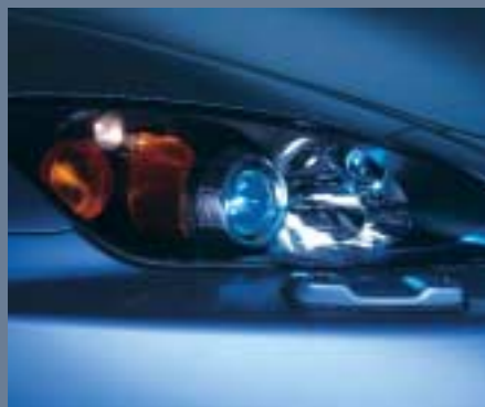
Triple beam projector headlamps providing powerful HID illumination in low light conditions, sit behind impact resistant, aerodynamic covers.
