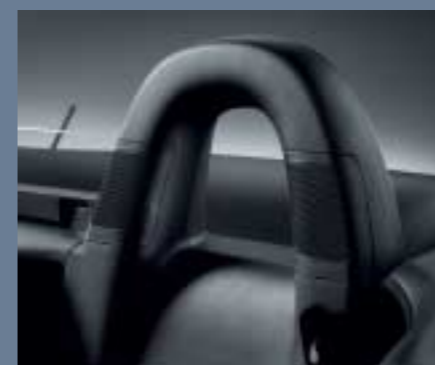
Roll bar speakers mounted in the headrests maximise sound quality with the roof down.
