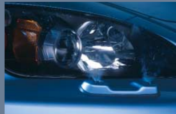
To ensure that the HID headlamps maintain their efficiency, powerful headlight washers are fitted as standard.
