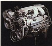
Z28 Coupe is available with a 5.7 Liter V8 with Tuned-Port Fuel Injection. Horsepower is 245 at 4400 RPM.
