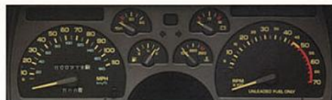
Camaro's standard analog gage package includes tachometer, trip odometer, voltmeter, temperature and oil pressure gages.
