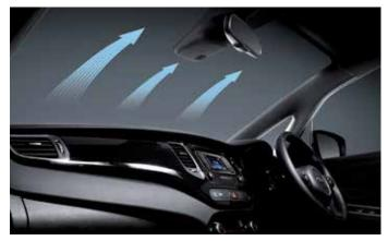
**Auto de-fogging system (special edition 'SR7' upwards)** – A sensor automatically initiates a de-fogging process when condensation is detected on the windows to ensure optimal visibility and to prevent humidity from building up on the windows.
