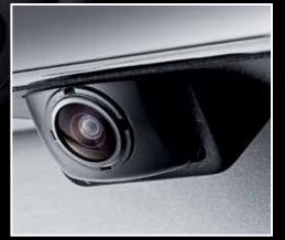
Reversing camera integrated into the centre fascia screen ('3' and '4' grades only) – The popular reversing camera feature is combined with reversing sensors which help minimise the collision risks involved when parking or manoeuvring. The rear camera view shows superimposed parking guidelines to assist the driver in easier, more effective parking. Reversing sensors are a standard feature on the special edition 'SR7' models upwards.
