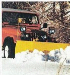
CJ snowplow—dealer installed
