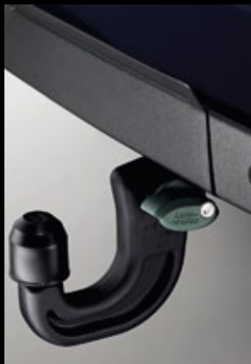
Quick Release Tow Bar KNB500070 Easily removed. Lockable for security. Tow bar height 400mm from ground. 3,500kg trailer load capacity (150kg trailer nose load).
