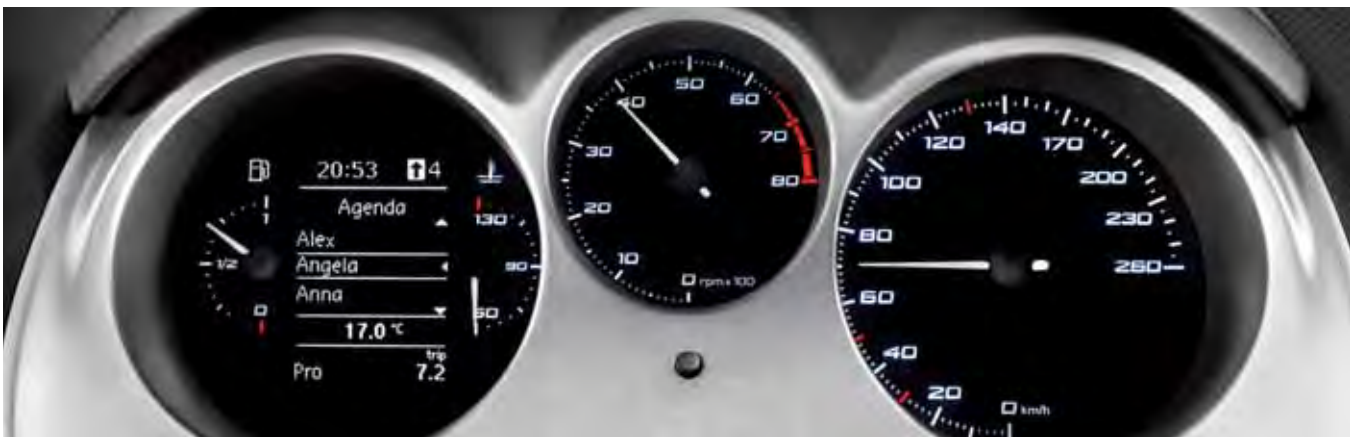
Instrument cluster with white graphics, showing the phone book function in the multi-function display (included in the optional Bluetooth® Communications Pack). A gearshift indicator ensures either a more sporty drive or maximum efficiency.
