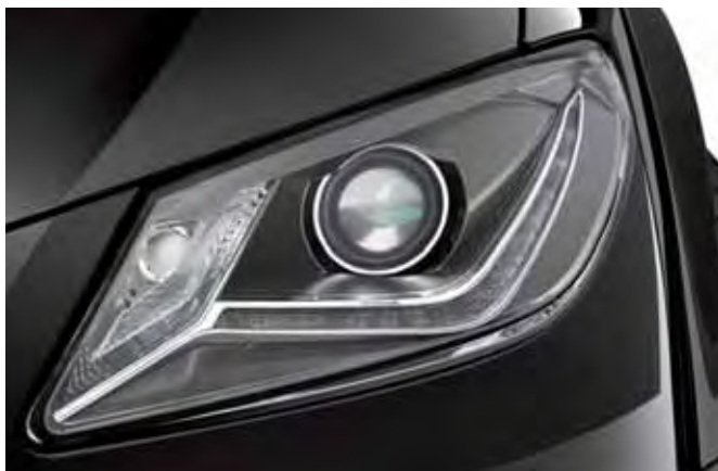
Bi-xenon headlights with LED daytime running lights, AFS, automatic range adjustment and headlight washer system.
