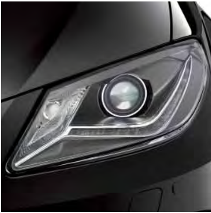
Bi-xenon headlights with LED daytime running lights, AFS, automatic range adjustment and headlight washer system. SE Sp
