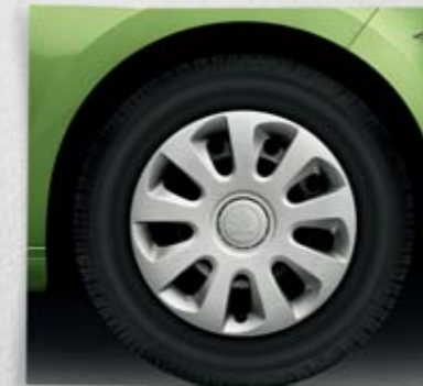
5.0J x 14" steel wheels for 165/70 R14 tyres with large Aries hub covers.
