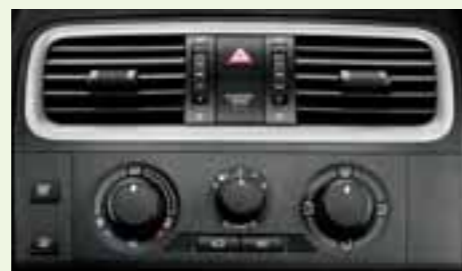
Climatic – air conditioning with automatic regulation and combi filter: automatic maintenance of preset temperature of the air inflow, manual regulation of air volume and setting of exhaust.
