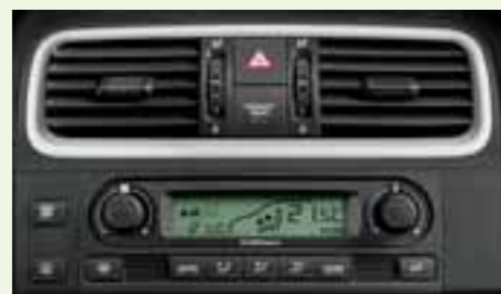
Climatronic – air conditioning with electronic regulation and combi filter: automatic maintenance of interior temperature, automatic regulation.
