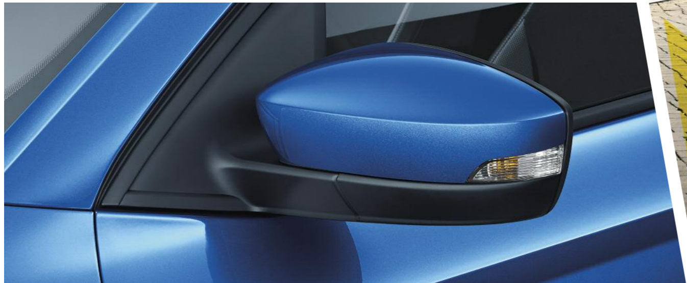
The side indicators have now been moved into the door mirrors creating a clean and sharp side profile.
