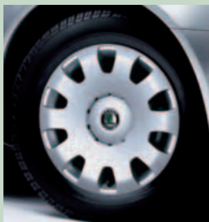
Steel wheels 6.0J x 15" with 195/65 R15 tyres and Drive hub covers.
