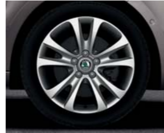
7.5J x 17" Trifid alloy wheels for 225/45 R17 tyres.
