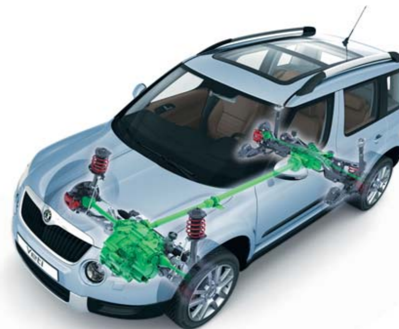
Škoda Yeti with a 4-wheel drive and a 4th generation Haldex clutch (1.8 TSI/118kW and 2.0 TDI CR DPF/81kW; 103kW and 125kW engines)
