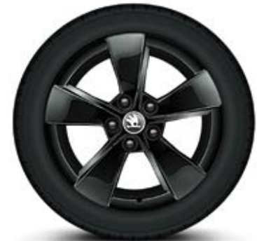
Leichtmetallräder 7,0 J x 17" «EREBUS» (Pneu 225/50 R17), in Schwarz; Yeti Outdoor
