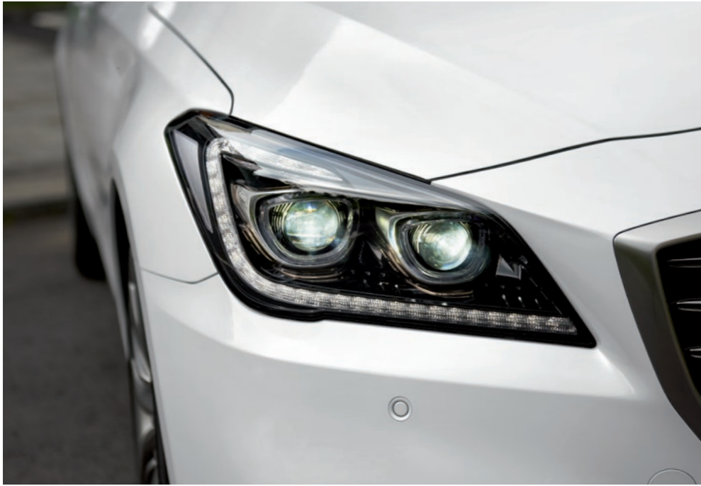
Full LED adaptive headlamps _ 3 dimensional headlamps convey Genesis G80's unique sensibility. Beam patterns adapt automatically to driving speeds and lane changes to widen the field-of-view and improve safety.
