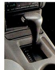
Below: An optional 4-speed electronically controlled automatic transaxle is offered on Taurus SHO with a 3.2 liter V-6 engine to maximize performance.
