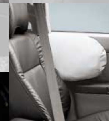
Standard on Outback Limited and Outback H6-3.0 models,* front seat side-impact air bags are mounted on the front seats, maintaining optimal placement regardless of seating position.**
