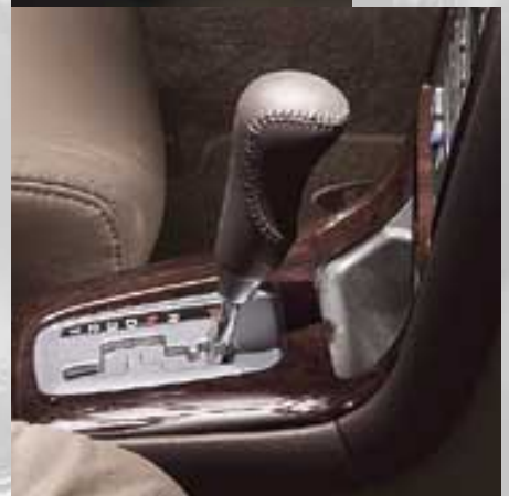
A 4-speed electronically controlled automatic transmission is standard in all Outback H6-3.0 models. The gated shifter provides precise control for manual gear shifting, if desired.
