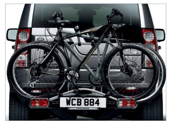
Tow Bar Mounted Two Bike Carrier VPLVR0067 – LHD (not shown) Three Bike Carrier VPLVR0069 – LHD (not shown) Fits to both Quick Release and Multi-Height Tow Bars. A trailer can not be towed at the same time. For further information on Land Rover Bikes please go to www.2x2worldwide.com
