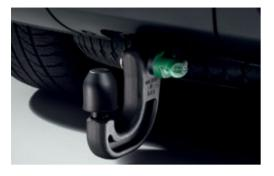
Quick Release Tow Bar\* LR040247 Lockable for security. Easily removed. 50mm/1.9 inches tow ball, height 400mm/15.7 inches from ground. 3,500kg/7,7/6/bs trailer load capacity (150kg/330.7/bs trailer nose load).
