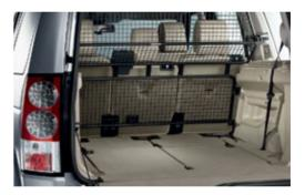
Cargo Barrier VUB501170 Easily removed. Retains cargo according to EC regulation 17. Can be fitted with Loadspace Rubber Mat (LR006401), Rigid Loadspace Protector (EBF500080) and used with standard loadspace cover.
