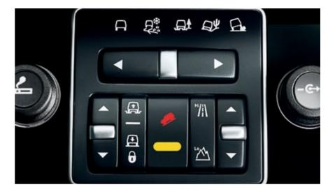
TERRAIN RESPONSE® SYSTEM. Optimises the vehicle set-up for virtually all on-road or off-road driving situations, with five different settings to suit different terrains such as Grass/Gravel/Snow, Sand, Mud and Ruts and Rock Crawl.
