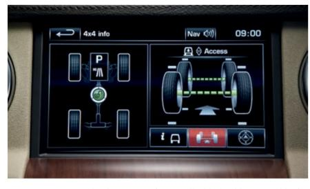
AIR SUSPENSION. Four-corner independent air suspension features variable ride height and electronic cross-linking for a constant level ride height irrespective of load distribution. Ride height can be raised up to 125mm to clear obstacles or lowered by 50mm for easy access and loading.
