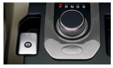
**ELECTRIC PARKING BRAKE (EPB).** A switch next to the eight-speed Drive Select is designed to electrically apply and release the parking brakes on the rear wheels. A simple pull of the lever applies the brake manually and a press releases it. The parking brake will also release automatically upon drive away.
