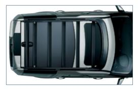
Expedition Roof Rack\* CAB500021PMA Vehicle must be fitted with a Short Roof Rail Kit CAB500120PVJ (not shown)/CAP500090. Vehicle height when fitted 2,100mm/83 inches at normal ride height. Maximum payload 54.3kg/1201bst.
