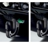
'N' and 'S' Type Towing Electrics\*\* VPLAT0011 Provides all trailer rear lighting and interior equipment power, where required. Supplied as a complete kit. Compatible with the Lighting Board (STC8153). 13 Pin Towing Electrics\*\* VPLAT0012 European-style towing electrics capable of supplying all trailer rear lighting and interior equipment power. Not compatible with the Lighting Board.
