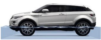
WADING DEPTH Maximum wading depth 500mm
