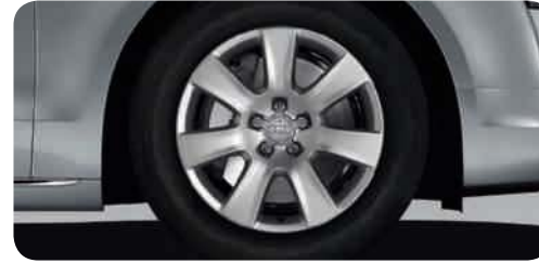
Cast aluminium winter wheels in 7-arm design size 7.5 J x 18 with 235/55 R 18 tyres 1 , permissible top speed 210 km/h, can be fitted with snow chains
