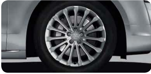
Cast aluminium wheels in 15-spoke design, partly polished 2 size 9 J x 19 with 255/45 R 19 tyres 1 (optionally available with run-flat tyres)
