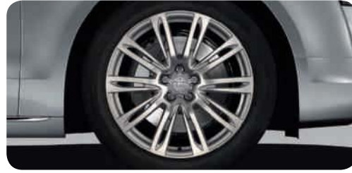
Forged aluminium wheels in 10-parallel-spoke design, partly polished 2 size 9 J x 20 with 265/40 R 20 tyres 1
