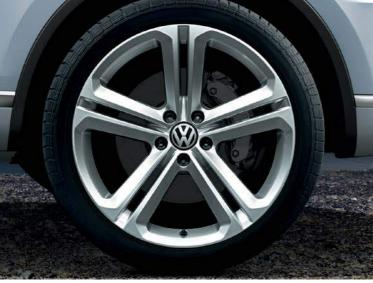
RLP SE RL 'Mallory' 9½J x 21 inch alloy wheels 275/40 R21 107Y low rolling resistance tyres and anti-theft wheel bolts.
