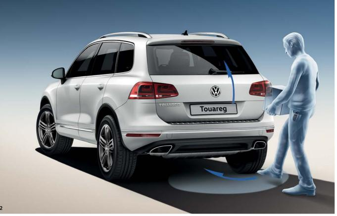
02 The hands free tailgate opening function enables you to open the tailgate without having to make contact with your Touareg as long as you have the key in your possession. A small foot movement triggers sensors at the vehicle's rear and the rear tailgate will open out. Hands free tailgate opening is a function of the optional keyless entry/keyless start and full electric tailgate operation. Optional on SE and Escape models.
