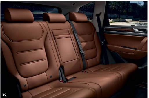
10 The modular design of the rear seating area enables each rear seat to be moved lengthways and the backrest inclined to three different angles. When moved forward, this increases the boot volume from 580 to 679 litres.
