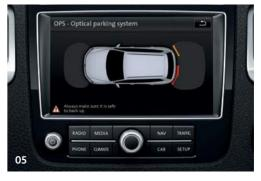
05 Parking sensors alert you with an optical and audible warning as soon as your vehicle approaches an object to the front or rear when manoeuvring into a parking space. A visual representation of how close the front or rear of the vehicle is to an object will also be displayed on the vehicle's radio system display. Standard on all models.
