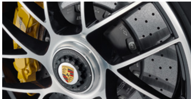
Porsche Ceramic Composite Brake (PCCB), 20-Zoll 911 Turbo S Rad
