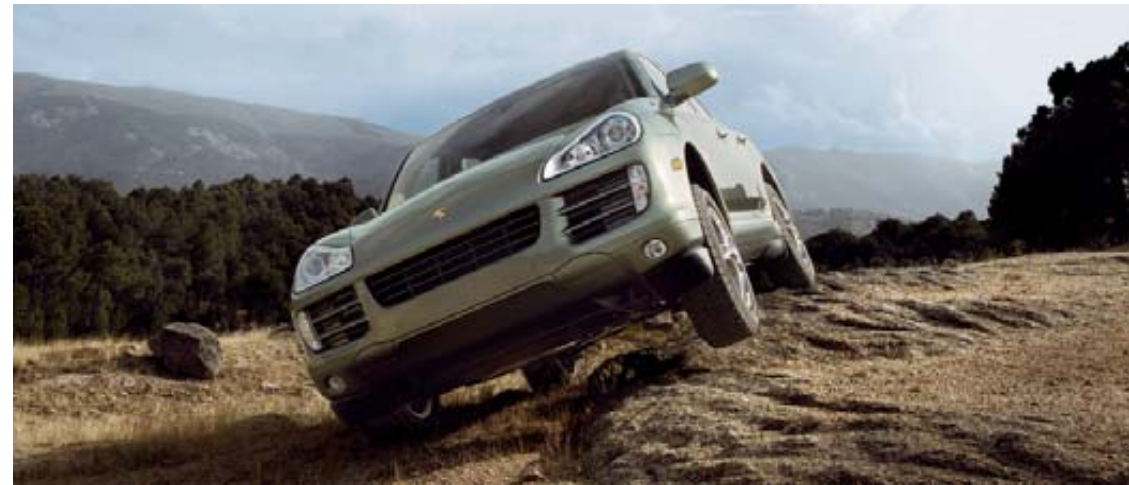
PDCC in On-road mode: reduced wheel articulation
