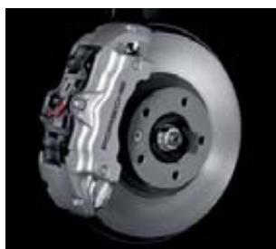
Cayenne S: standard front brake with 13.78-in. disc
