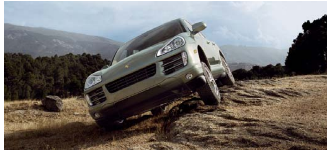
PDCC in Off-road mode: increased wheel articulation
