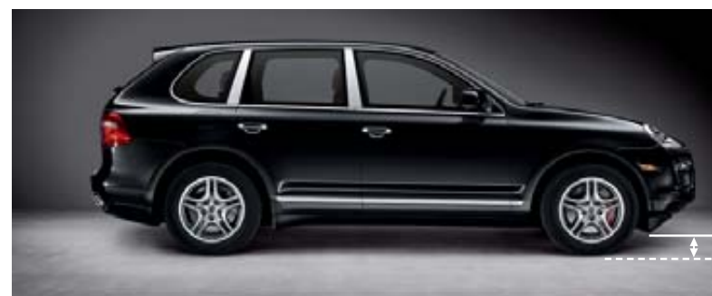
Loading Level: 6.34 inches
