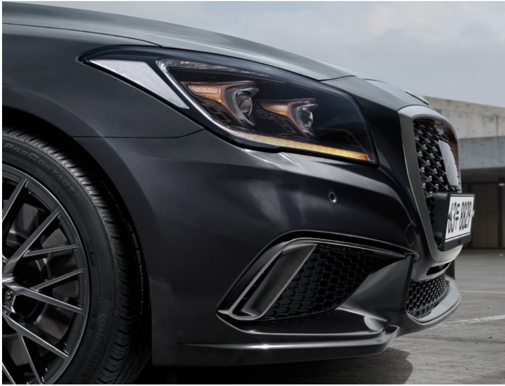
Sequential turn signals & Full LED adaptive headlamps _ Turn signals light up sequentially and headlamps feature prominent copper chrome details. Vertical air curtains below headlamps improve aerodynamic and brake-cooling performance.
