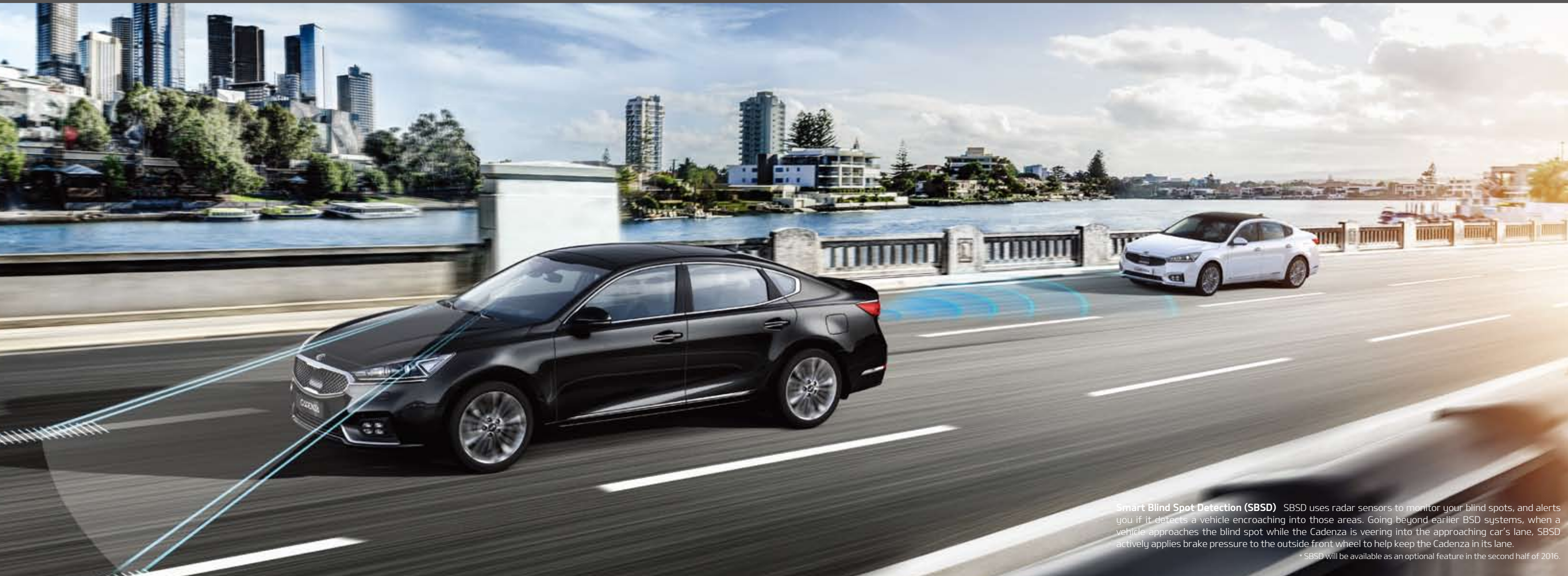
Lane Change Assist (LCA) LCA issues visual alerts on the side mirrors if it senses a vehicle approaching rapidly from behind in adjacent lanes.
