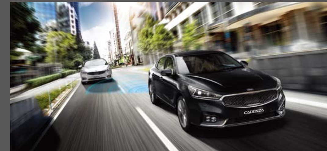
Lane Change Assist (LCA) LCA issues visual alerts on the side mirrors if it senses a vehicle approaching rapidly from behind in adjacent lanes.
